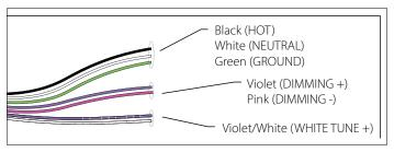
SpectraSync Tunable White luminaires are provided with two 0–10V circuits. The violet and pink circuit is for wiring to any qualified 0–10V controller for dimming. The violet/white and grey/white circuit is for wiring to any qualified 0–10V controller for Tunable White CCT control.
