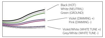
SpectraSync Tunable White luminaires are provided with two 0–10V circuits. The violet and pink circuit is for wiring to any qualified 0–10V controller for dimming. The violet/white and grey/white circuit is for wiring to any qualified 0–10V controller for Tunable White CCT control.
