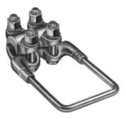
Aluminum alloy stirrup clamp for making temporary or permanent ground connections to aluminum tubing. The copper stirrup loop is tin plated and is compressed into the body costing.
