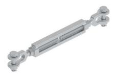
"Turnbuckles are used as adjustable extensionlinks to maintain proper tower clearance onassemblies at tower end. Jaw ends are supplied with bolt, nut, andhumpback cotter pin. Add "LN" suffix if jam nuts are required."
