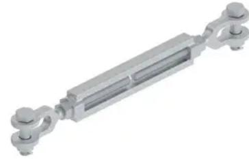
Turnbuckles are used as adjustable extension links to maintain proper tower clearance on assemblies at tower end. Jaw ends are supplied with bolt, nut, and humpback cotter pin. Add "LN" suffix if jam nuts are required. Remove "BNK" suffix for type EE turnbuckles.
