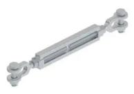
Turnbuckles are used as adjustable extension links to maintain proper tower clearance on assemblies at tower end. Jaw ends are supplied with bolt, nut, and humpback cotter pin. Add "LN" suffix if jam nuts are required. Remove "BNK" suffix for type EE turnbuckles.
