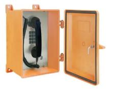
Model 354-001 Series NEMA 4X Telephones are designed for use in extreme weather conditions where temperature and moisture are a concern. They are ideal for use in areas that require a direct water spray (hose-down) for cleaning purposes or where a noncorrosive material is required. The 354-001 Series Telephone is perfectly suited for areas considered too harsh for a standard telephone.
