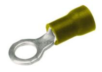
Copper Terminal, Ring Tongue, 12-10 AWG, 1/4" Stud, Vinyl Insulated, Tin Plated.
