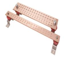
Cu Bus Bar, 22 Holes, 10 in L, 4 in W, 1/4 in T,Can be used as a common ground point and power applications as well.
