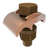
Accommodates: Bar: 1/4" - 1'; Cable: 2/0 SOL - 250 kcmil Copper; Suitable for Grounding and Direct Burial Bonding Equipment.
