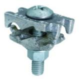
Cast Copper Alloy Cable Tray Ground Clamp, #6 Sol. (.162 Dia.) -1/0 Str. (.372 Dia.), 1.12 in L, 1.45 in W, Tin Plated.
