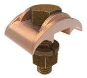
Mechanical Grounding Connector, 2 Cables to 1/4" Thick Bar, 2/0 AWG (Sol) -250 kcmil, 1/2" Stud, 2.07 H.
