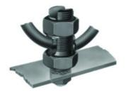
Tin plated; Accepts 2 conductors; #2 - 2/0 Stranded Copper; #2 - 3/0 Solid Copper; 1/2" Stud.
