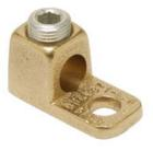
Copper Terminal, 1 Hole, 14 AWG (Sol)-4 AWG (Str), 1/4" Stud, 1 Screw.
