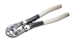
Splices and Terminals: #10 str. to 4/0 ACSR; Installs Splices, Taps or Terminations: #8 to 500 kcmil Copper Stranded, #8 to 350 kcmil Copper Flex, #8 to 350 kcmil Aluminum
