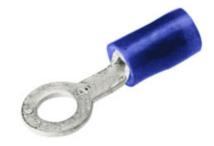
Copper Terminal, Ring Tongue, 16-14 AWG, #6-#8 Stud, 600 Volts Max., Nylon Insulated, Funnel Entry, Tin Plated.
