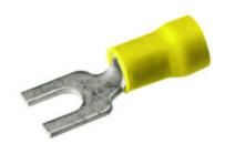
Copper Terminal, Fork Tongue, 12-10 AWG, #8-#10 Stud, Vinyl Insulated, Tin Plated.
