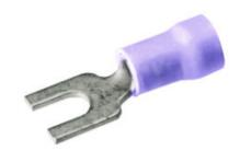
Copper Terminal, Fork Tongue, 16-14 AWG, #8-#10 Stud, Vinyl Insulated, Tin Plated.
