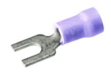
Insulated Brazed Fork Terminal, Insulated Brazed Fork Terminal, Smooth Entry, #16-#14, 600V, #3-#6 Stud, Vinyl Insulated, Tin Plated.
