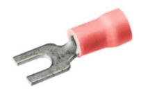
Fork Tongue Copper Terminal, 22-16 Max. Insul. Dia. Accom.: .145 Color Code: Red, 8-10, .95 in L, .41 in W, Polyvinylchloride Insulation.
