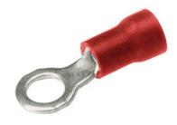
Terminal-Polyvinylchloride Insulated, Ring Tongue, 22-16 Max. Insul.Dia. Accom.: .145 Color Code:Red, 12, 1/4, 0.99 in L, .40 in W.
