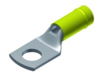
Ring Tongue Copper Tubing Terminal, Code: Yellow, #6-#8 stud, 1.14 in L, .37 in W, 300 Volts Max., 105 Deg C Max.
