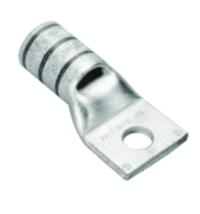
Copper Compression Lug, Ring Tongue, 1 Hole w/ Inspection Hole, AN-5 Flex/ AN-6 Flex,  $1\!/2''$  Stud, Short Barrel, Electro-Tin Plated.
