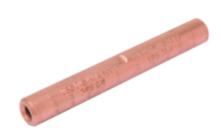
CU loop splice connector designed to withstand jumper loop tensile and vibration stresses up to 60 percentage RBS, 3-1/4 IN L.
