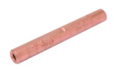
HYSPLICE Single Sleeve Full Tension Splice, Accommodates Wire: 8A COPPERWELD, Die Index: 162 or 202, Made of copper tubing, Installed with standard tools and dies.
