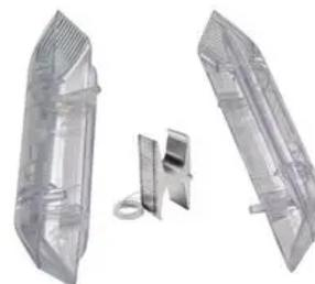
Copper Compression H Tap, Tin Plated, Accommodating the following wire sizes - Run (Main): 250 kcmil-2 AWG Class B,C, 4/0 AWG-2 AWG Class I, DLO; Tap 1: 8 AWG-14 AWG Class B, C, 8 AWG-14 AWG Class G,H,I, DLO, 8 AWG Class K, Tap 2: 8 AWG-14 AWG Class G,H,I, DLO, 8 AWG Class K, kitted with clear cover. See sale drawing for metric wire size accommodates
