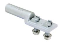
Disconnectable Terminal (With Fixed Hardware), 397.5 (26-7, 30-7) 477 (18-1) ACSR 477 (19, 37) 500 (37, 61) Al, 7-1/4 in L.
