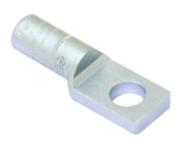
Al Compression Terminal, 1 Hole, #2 AWG ACSR, #1 - #2 Str Al/Cu, 0.56" Hole Dia., Tin Plated.
