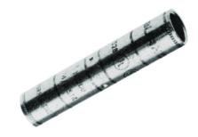
4/0 AWG CU, Long Barrel, Internal Chamfer, Tin Plated, UL/CSA, 90°C, Up to 35kV, PURPLE Color Code, 15 Die Index.
