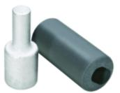
Aluminum Compression Pin Adapter, 1/0 AWG, 0.29" Plug Dia, 0.84" Plug Length, Al/Cu Rated, Tin Plated.
