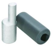
Aluminum Compression Pin Adapter, 4/0 AWG, 0.42" Plug Dia, 1.22" Plug Length, Al/Cu Rated, Tin Plated.
