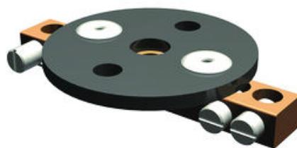
BONDIT® Intersystem Bonding Connector, #8 - #2 AWG Servit post #14 - #6 AWG Bus Bar, 2.92 in L, 2 in W.
