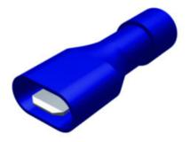
Fully Insulated Brass Male Disconnect, 16-14 AWG, Nylon Insulated, Funnel Entry, Tin Plated.
