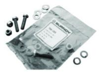
Stainless steel Hardware Kit, 2 Nos each 3/8" - 16 x 1.50" Long Hex SS Bolt (38X150HSSB), SS Hex Nut (38CHXNT), SS Split lock washer (38SWSSMD), 4 Nos SS Flat washer (38FWSS).
