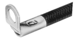
Copper Compression Right Angled Lug, Heavy Duty, 1 Hole W/ Inspection Hole, AN-2, 5/16" Stud, Short Barrel, Nickel Plated.
