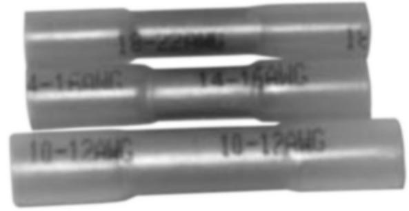
Cu Heat Shrink Butt Splice, 14-16 AWG, 1.50" L, Serrated bbl, Tin plated, For Use On Cu Cond.
