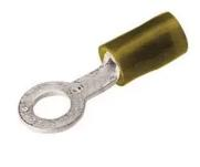
Copper Terminal, Ring Tongue, 12-10 AWG, 5/16" Stud, 600 Volts Max., Nylon Insulated, Funnel Entry, Tin Plated.
