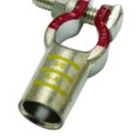
Battery Post HYDENT Cu Terminals, 4/0 AWG, 2.36" L, 1.02" W, Yellow, Wire Strip Length - 1-3/32" L.
