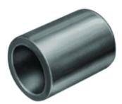
16,910 - 26,890 Circular Mils, CU, Internal Chamfer, Tin Plated, UL/CSA 90° Up to 35kV, Blue Color Code, 7 Die Index.
