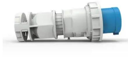
Heavy Duty Products, IEC Pin and Sleeve Devices, Male, Plug, 100/125 A 120/208 VAC, 4-POLE 5-WIRE, Blue, Watertight
