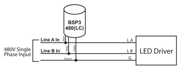
A single phase input from a 3-phase system uses only 2 phase line connections (A-B, B-L or C-A)
