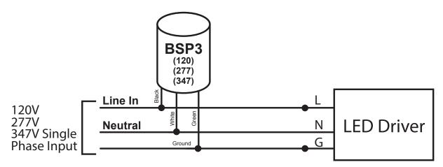
BSP3 and driver voltage must match input voltage
