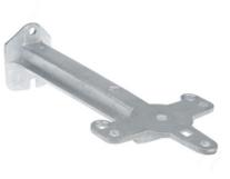
Equipment or Insulator Bracket, can be used for mounting pin or post insulators, cutouts, arresters or cable terminators. Can also be used for in-line deadend takeoffs. 18" extension from pole.
