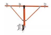
Mechanical Ratings:Max. Total Load: Balanced Vertical Load: 1000 lb.\* Unbalanced Vertical Load: 800 lb.Rated working load (per wire holder): Vertical with braces: 200 lb.\* Vertical without braces: 150 lb.\* Side Load: 100 lb.
