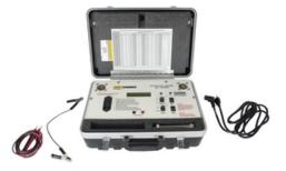
Self-contained, portable, convenient 120 VAC tester provides an easy way for an electric utility to check the resistance in protective grounding sets used by line personnel.
