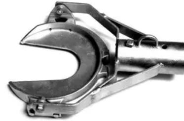
LINK STICK, SUSPENSION 1 1/2 X 7 FT, The Suspension Link Stick is designed for use on conductors from 1" to 2.5" diameter and can be used with various types of takeup devices at the structure end. The lip of the hook, actuated by an eye screw, swivels to accommodate various conductor sizes. The maximum load is 6,500 pounds.
