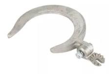
The self-aligning shepherd hook is designed for pulling and lifting insulator strings. Swivel action permits it to rotate and maintain its alignment with the insulator at all times. Heat treated aluminum alloy.
