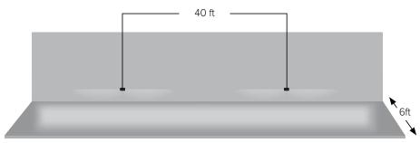
Recommended spacing's based on requirements for meeting the Life Safety Standard minimum illuminance of 0.1 fc and average illuminance of 1.0 fc. Assumes that the fixtures are wall mounted 18' above the floor in a corridor 6' wide with 8' ceiling height and reflectances of 80/50/20
