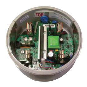
The Aclara DSI provides a simple way to connect and reconnect power customers. The switch manages power delivery to seasonal and rental properties, locations where utility-worker safety is a concern, and homes or businesses previously disconnected for nonpayment. The DSI eliminates service calls to turn power on and off — saving the utility time and money.
