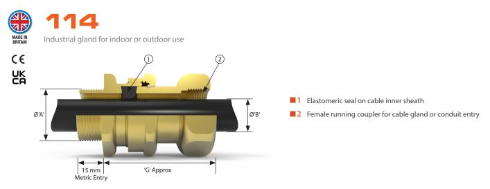
The 114 industrial cable gland offers a female running coupler and a seal onto the cable outer sheath for use with non-armoured elastomer and plastic insulated cables installed in conduit. May also be used with braided cables under certain conditions - See technical section for installation rules and regulations.
